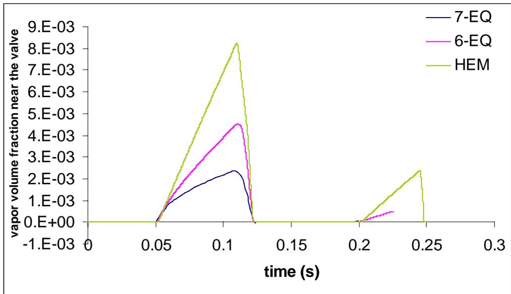
Fig. 1: Comparison of the 3-eq.-HEM, 6-eq. and 7-eq. models: temporal development of the vapor volume fraction at the point where the cavitation starts.
