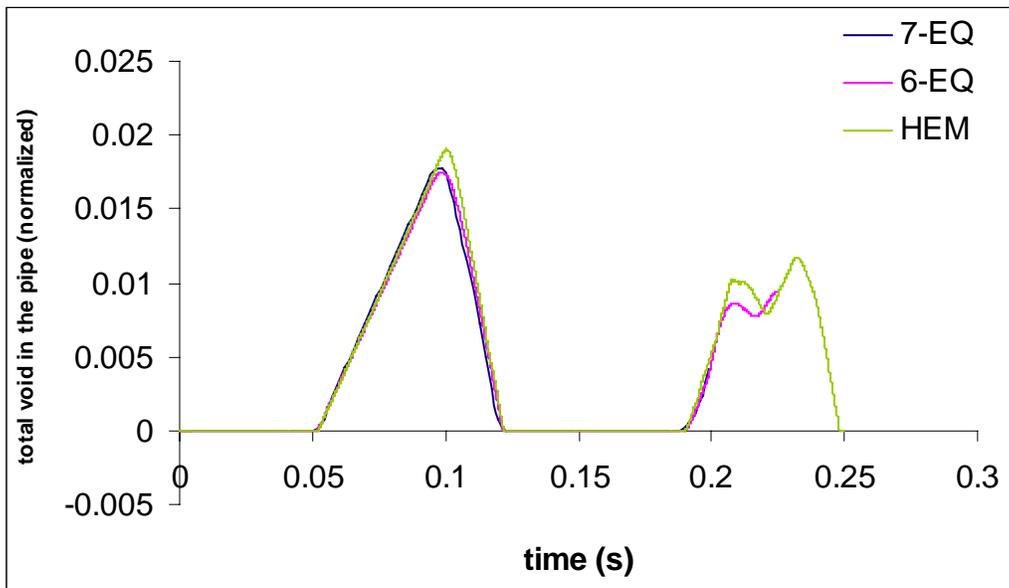
Fig. 3: Total volume of vapor created in the pipe predicted by the 3-eq., 6-eq. and 7-eq. models.
