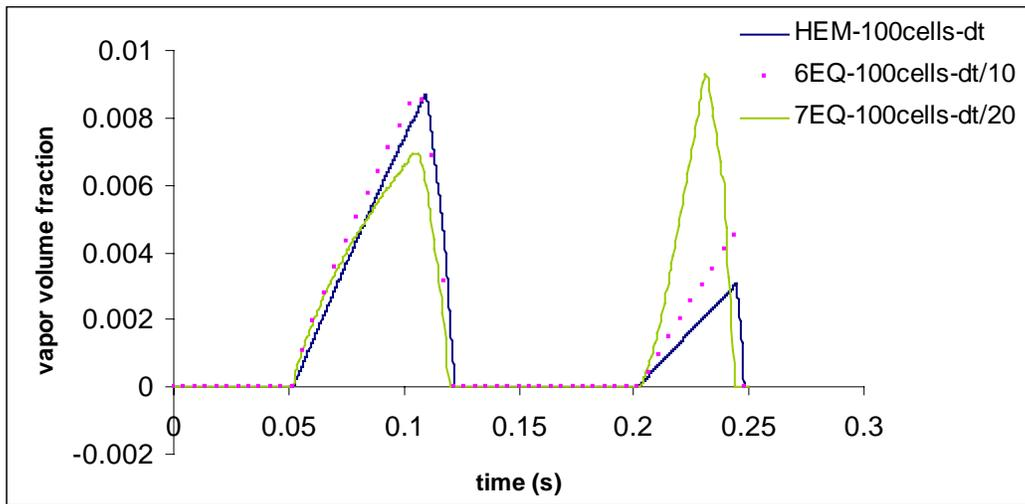
Fig. 4: Comparison of the 3-eq.-HEM, 6-eq. and 7-eq. models: temporal development of the vapor volume fraction in the point where the cavitation starts - the same grid but different time steps.
