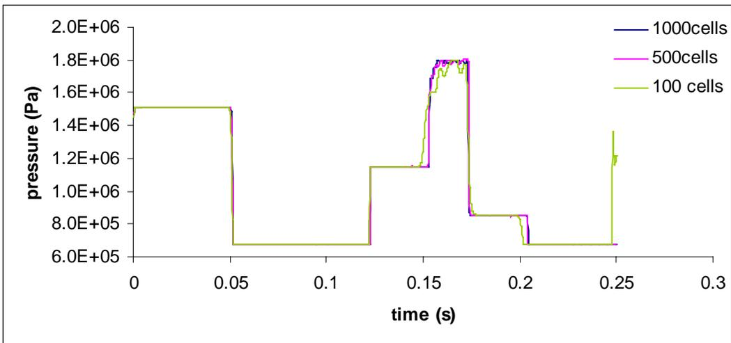
Fig 6: Grid refinement study performed with the 3-eq.-HEM model.
