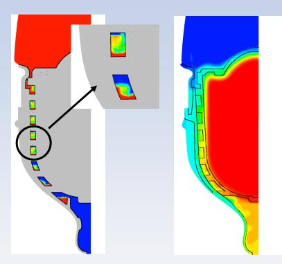
An accurate prediction of the first drop temperature and the pressure variations inside the channel required
