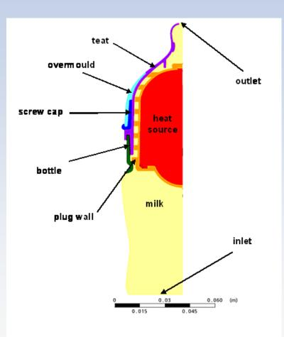
Modelling fluid and heat flow in such device is challenging:
