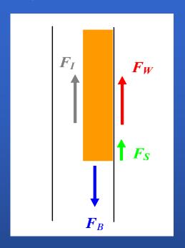
$$F_{B} = \rho_{milk} g \left( z_{0} + \frac{h_{plug}}{L_{channel}} x \right) \left( w_{milk} h_{channel} \right)$$
