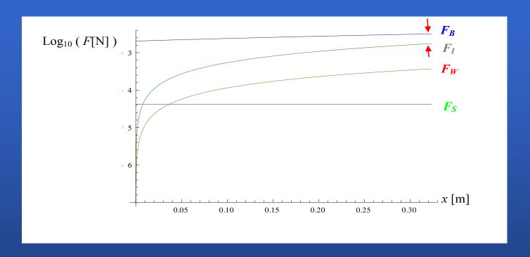
In order to prevent occurrence of slugs (i.e. to maintain smooth milk flow) a force balance was analysed taking into account buoyancy force (F<sub>B</sub>), wall friction (F<sub>W</sub>), interphase drag (F<sub>I</sub>) and surface tension force (F<sub>S</sub>)
