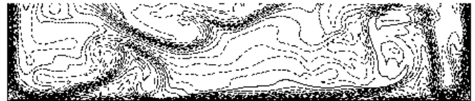
Figure 11: Unsteady temperature field at lower boundary, Ra=10^{11} , Pr=0.8
