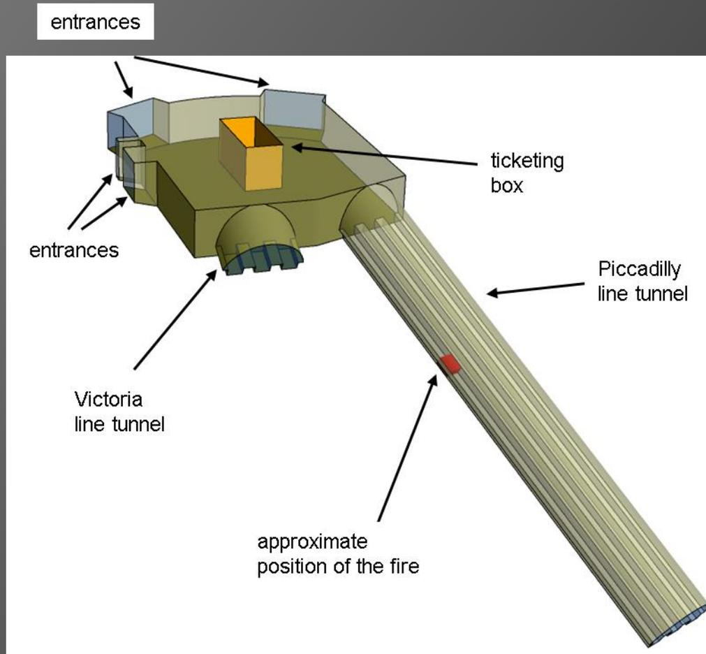
CFD simulation domain for the King's Cross accident simulation [8]
