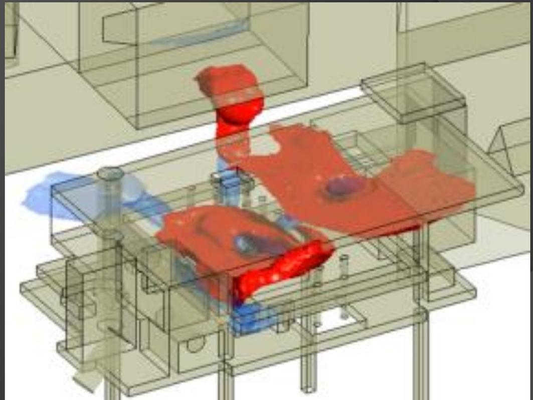
Premixed combustion developing into jet fire
